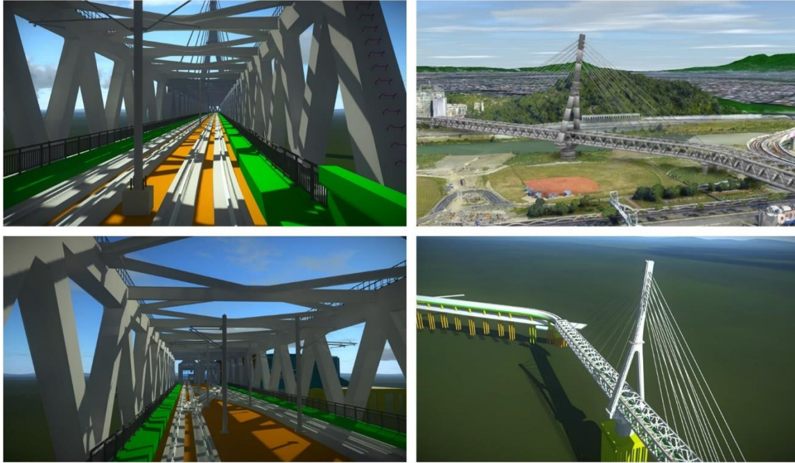
374 375 Figure26: The BIM output for the steel truss frame of the Anhsin Bridge (AB).
